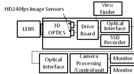
Fig. 11. Block diagram of HFR 3D Camera
