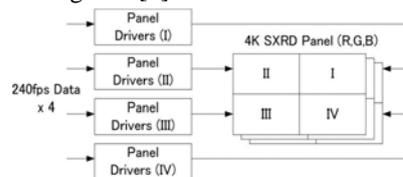
Fig. 12. Block diagram of the interface of the customized 240fps 4kx2k projector
