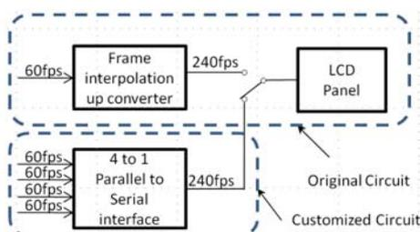
Fig. 13. Block diagram of the interface of the customized 240fps LCD Monitor
