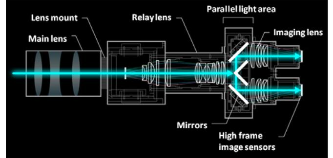
Fig. 5. Optics of HFR 3D Camera
