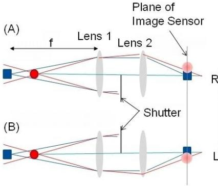
Fig. 4. Conventional single lens 3D system
